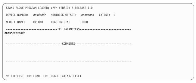
Figure 8. Sample Stand Alone Program Loader Panel
